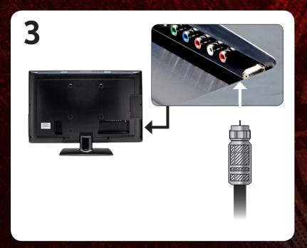
If you have an external antenna or a cable connection that extends from a wall outlet, connect it to the TV with an RF/Coaxial cable.
